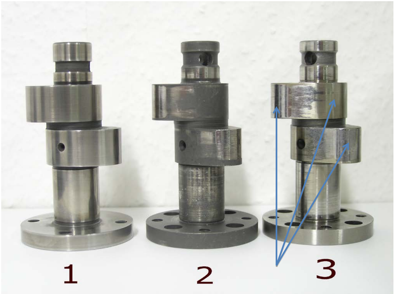
Camshaft: New (1), used one without RVS (2), used camshaft treated with RVS (3). The triboceramic surface produced by RVS Technology can be seen with naked eye (arrows).
