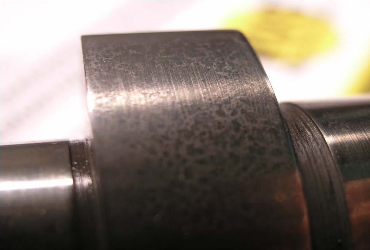
Picture 1. New cam. The surface structure of a new cam after machining. The micro relief is destroyed.
